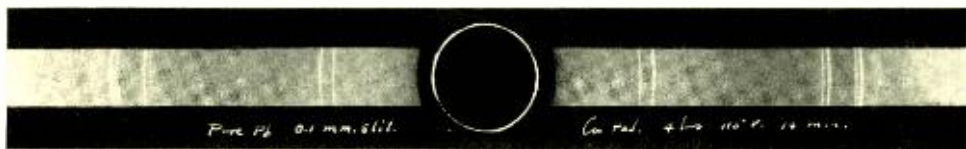
Fig. 5—Reflections from lead photographed in an X-ray camera which has been arranged as illustrated in the photograph of Figure 4
