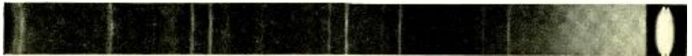
Fig. 2—X-rays from copper reflected by crystalline silver. The K\alpha double is separated at the left, where the angle of reflection is almost 80^\circ . This illustrates the high dispersion obtained for large angles of reflection
