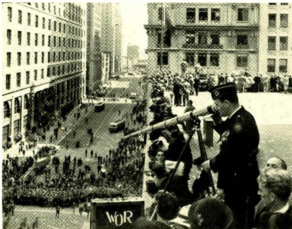
Sgt. Harry P. Goodwin, of American Legion Post 25, New Jersey, trains the Laboratories' "machine gun" microphone upon a brass band passing below the Empire State Building. An unusually successful broadcast of a difficult subject was accomplished by this experimental Western Electric device, which picks up a maximum of sound from the object upon which it is trained, but shuts out to a great extent sounds from other sources
