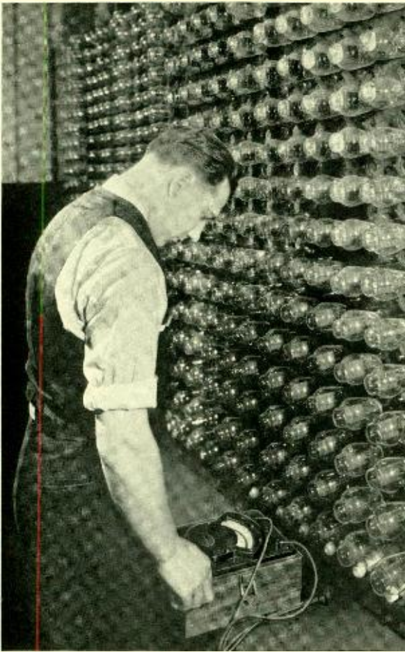
Fig. 5—L. G. Petrovich checking operating conditions of 300A vacuum tubes on life test
