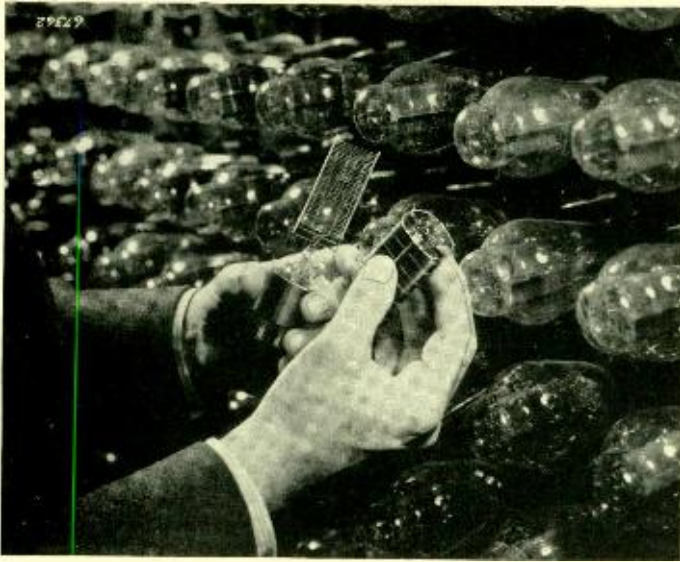
Fig. 1—Disassembled elements of the 300A tube against a background of the same tubes on life test
