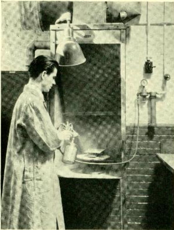
Fig. 1—Wood and metal panels are prepared for exposure by the same finishing procedure as that used in painting automobiles
