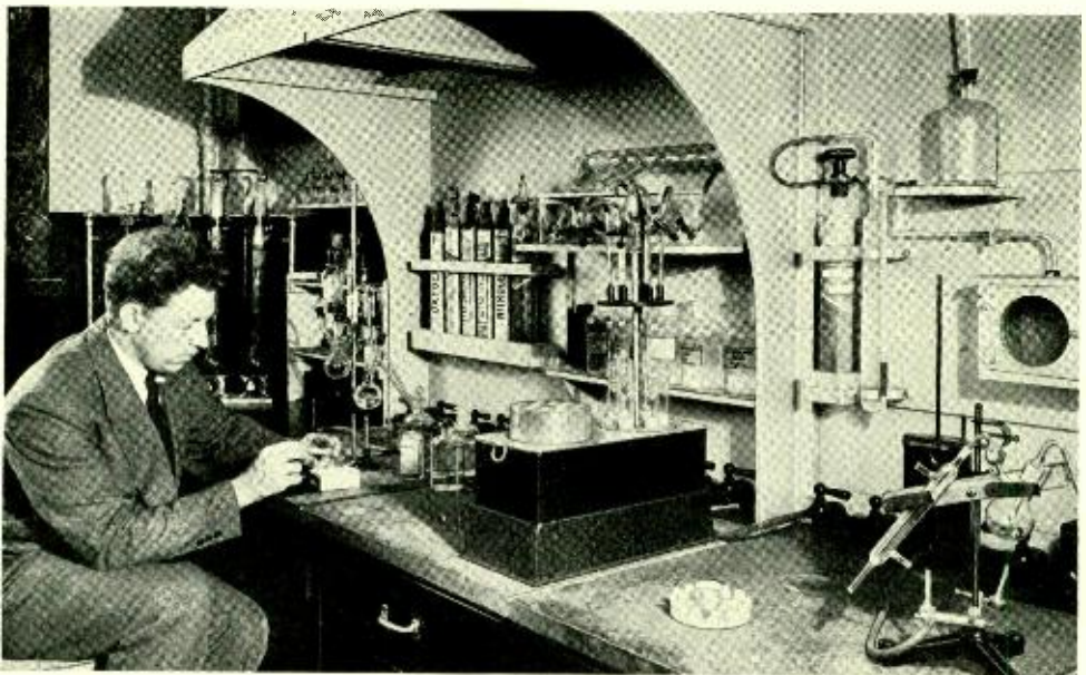
H. W. Hermance, in the microchemical laboratory, prepares apparatus for a determination of minute quantities of arsenic
