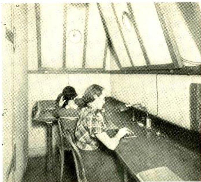
Fig. 2—Each observer presses keys corresponding to the three sounds of the syllable as she understands them
