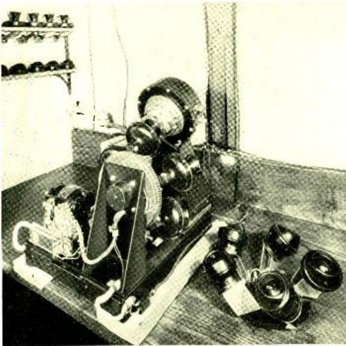
Fig. 5—The transmitters used in testing are mounted on a motor driven disc which is under the control of a dial on the control panel. This apparatus serves to agitate the transmitters in a uniform way and then center them properly in front of the artificial mouth
