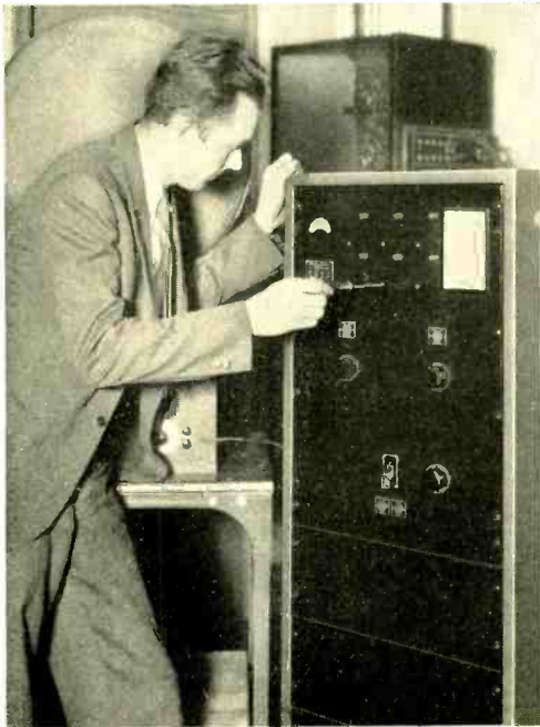
Fig. 1—The 11B receiver, like the 11A, mounts in the 6A cabinet, which is rugged and self supporting
