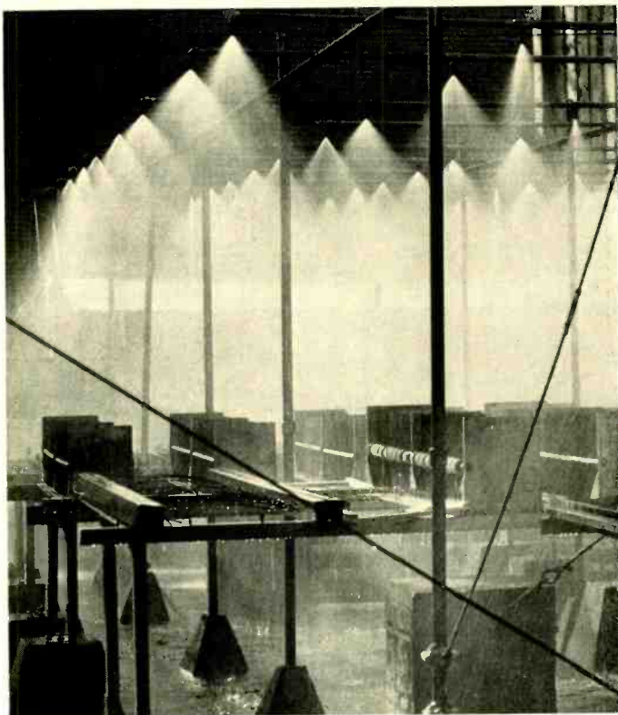
Fig. 3—One of the more spectacular uses of water in these Laboratories' research is in the accelerated corrosion tests on the roof of Section G
