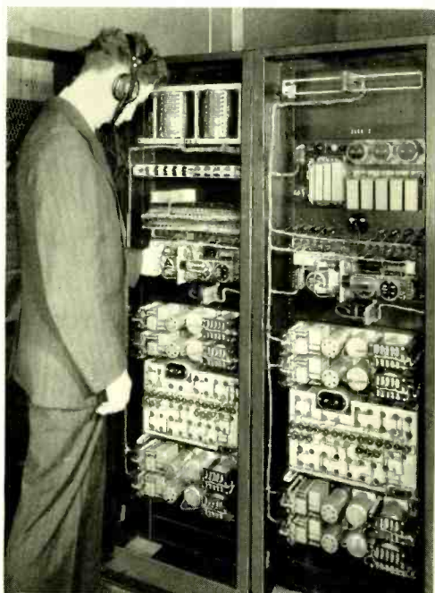
Fig. 3—The amplifiers and equalizers for the binaural system were adapted for use at the Century of Progress Exposition by L. B. Cooke
