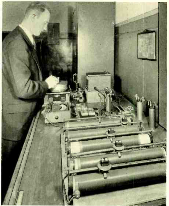
Fig. 2—As formerly set up, the circuit employed slide wire rheostats and the complete equipment covered the entire surface of a large table
