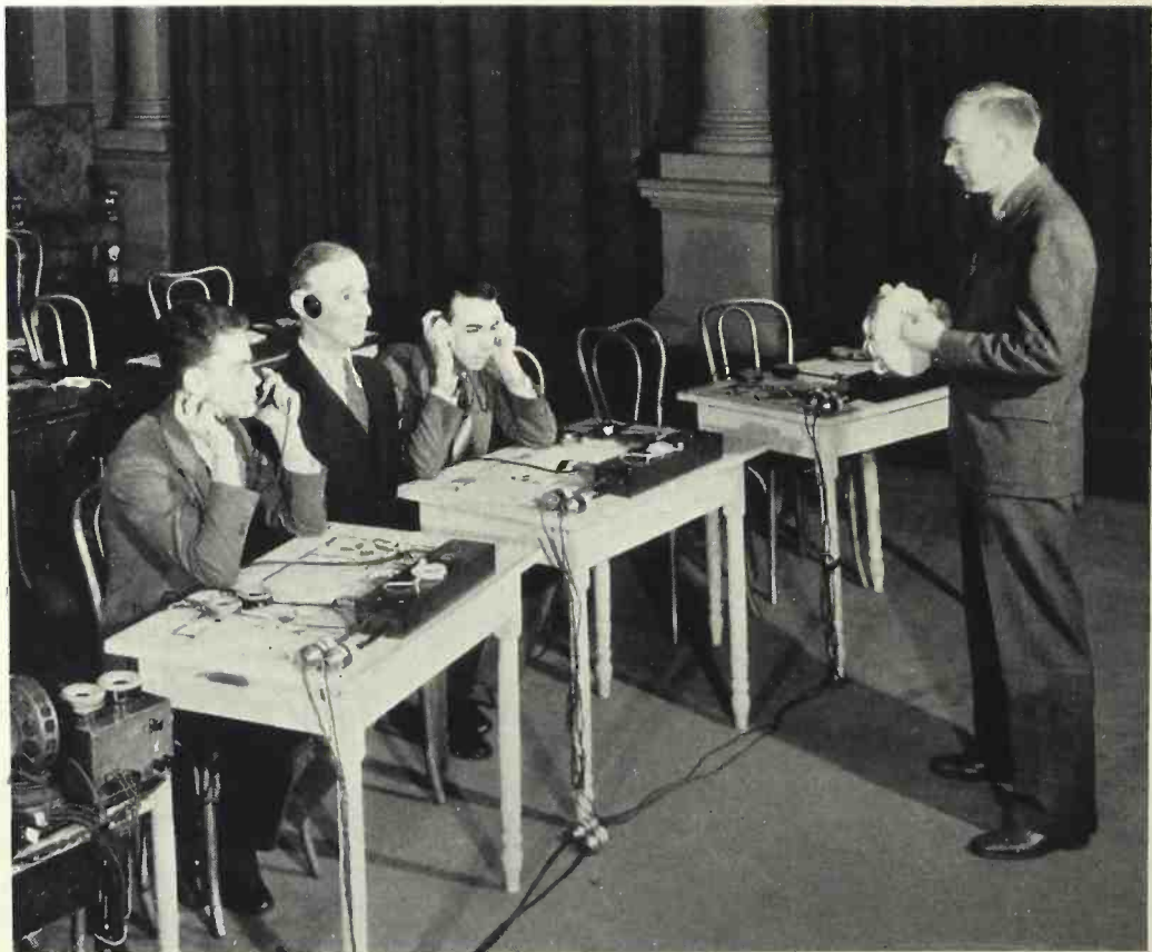
Seated alongside the microphones which are placed in the head of the tailor's dummy, these observers listen to the jingle and thump of a tambourine, and compare transmission through the air and through the microphone system
