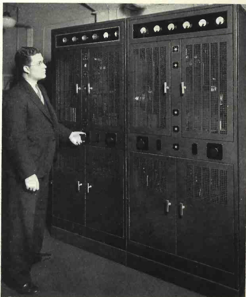
Fig. 7—1000 watt broadcast unit. Transmitter at left and amplifier on the right
