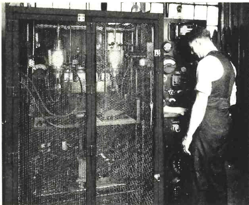
Fig. 3—All tubes are exhausted on a special high-vacuum system and during the process the metal parts are heated to rid them of occluded gases
