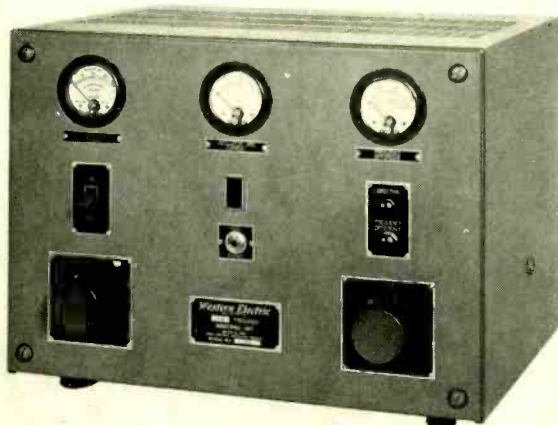
Fig. 2—The amount of departure of the station from its assignment can be read directly on the right-hand meter
