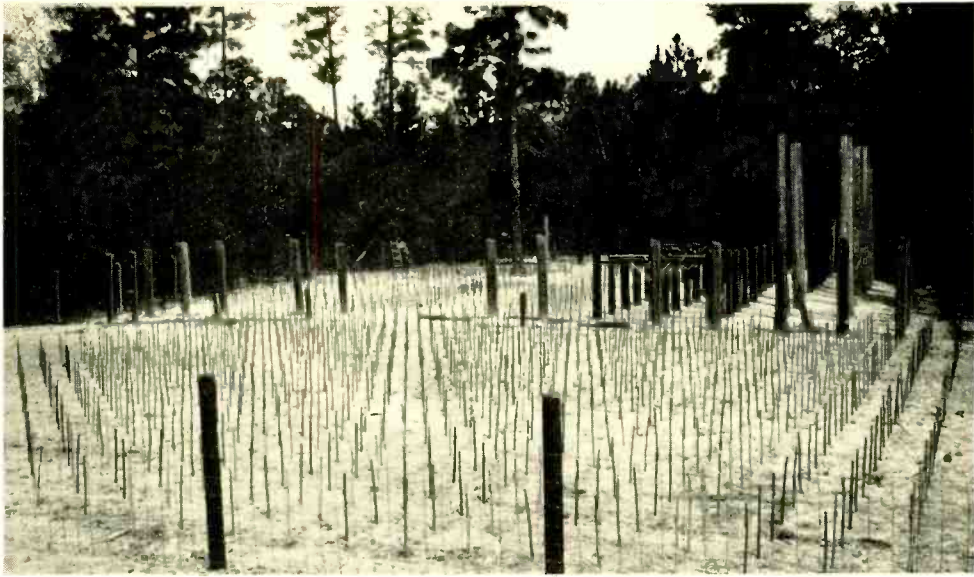
Fig. 3—The sapling plantation affords an accelerated testing ground for wood preservatives
