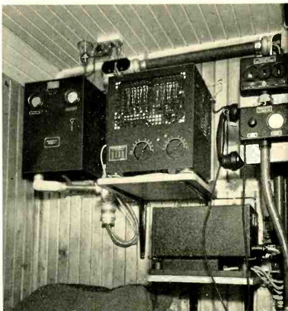
Fig. 2—An installation of harborcraft radio on a trawler out of Boston
