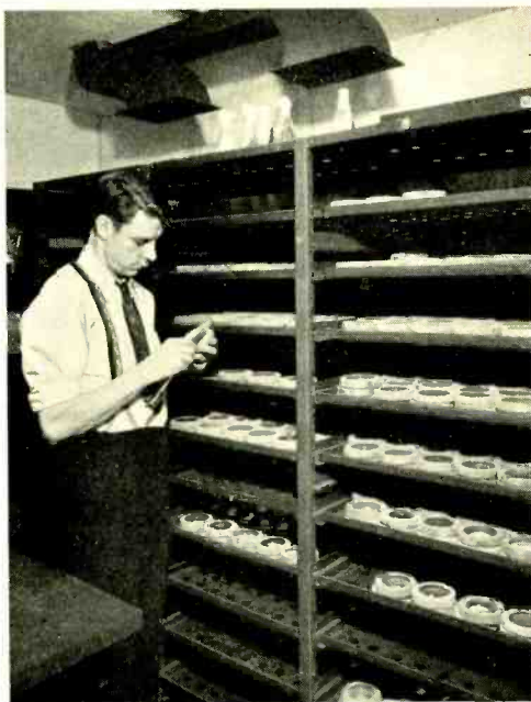
Fig. 2—The toxicity of a preservative is determined by observing the rate of growth of different fungi in cultures containing different concentrations of the preservative
