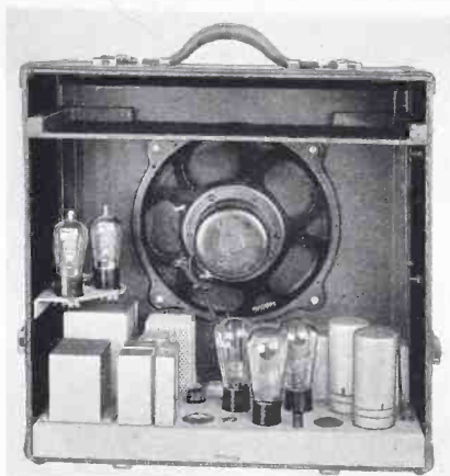
Fig. 2—Amplifier and loud speaker are combined in a single unit. The rear cover is removed as shown while the set is in operation to provide ventilation
