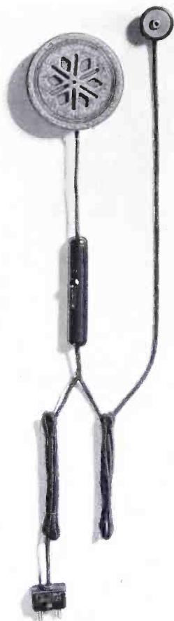
Fig. 3—The 36-A audiphone employs no amplifier but has a wide field of use with those whose hearing is only moderately impaired
