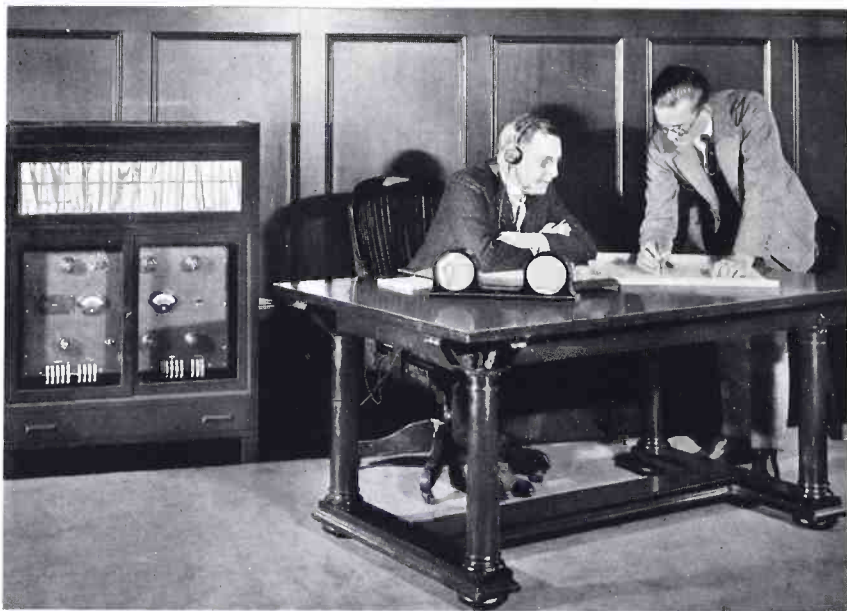
Fig. 1—Although the 10-A audiphone was very satisfactory as a hearing aid, it was far too large for general use
