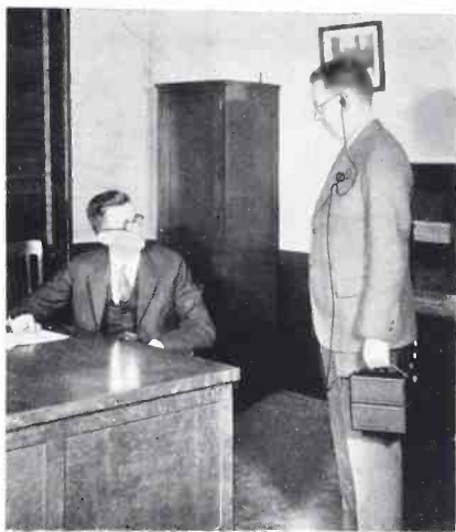
Fig. 2.—In the 6032 audiphone a great reduction in size was obtained but even with it the most desirable size did not seem to be reached
