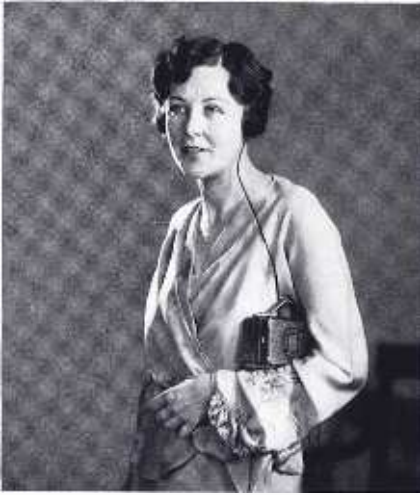
Fig. 6—Still another alternative arrangement is provided by the 12-A carrying case which assembles the complete 38-A audiphone and battery in a single unit
