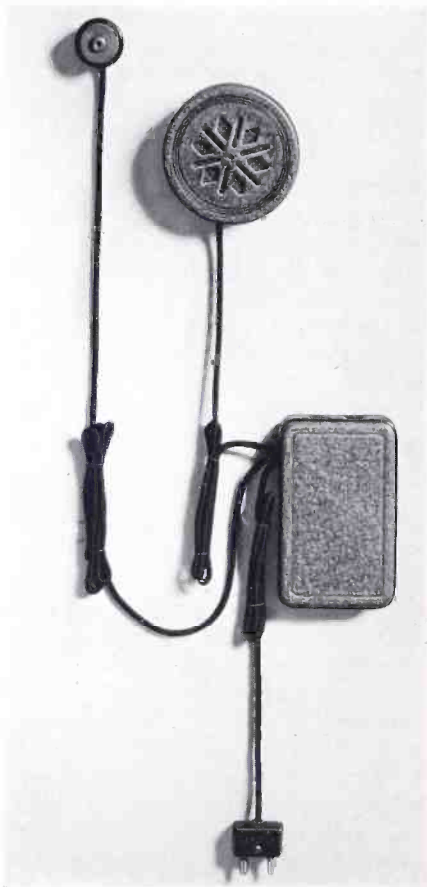
Fig. 4—The 37-A audiphone has an amplifier, but mounted with the rheostat in a box of cigarette-case size, it makes little more demand on space than does the 36-A
