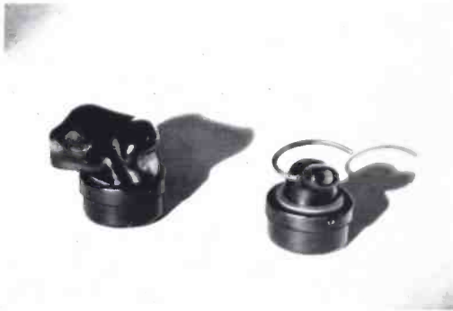
Fig. 2—The universal type earpiece, on the right, may be adjusted to conform to the ear, while the individual type, on the left, is specially moulded for each user
