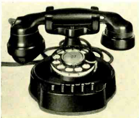
Fig. 1—Three trunk buttons, a hold, and a local button are mounted in the applique base of the hand-set used with the 750-A PBX
