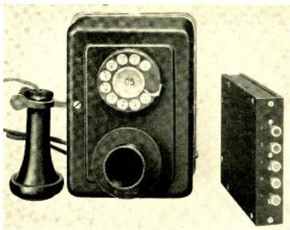
Fig. 2—A separate key is arranged for use with desk stands or wall sets
