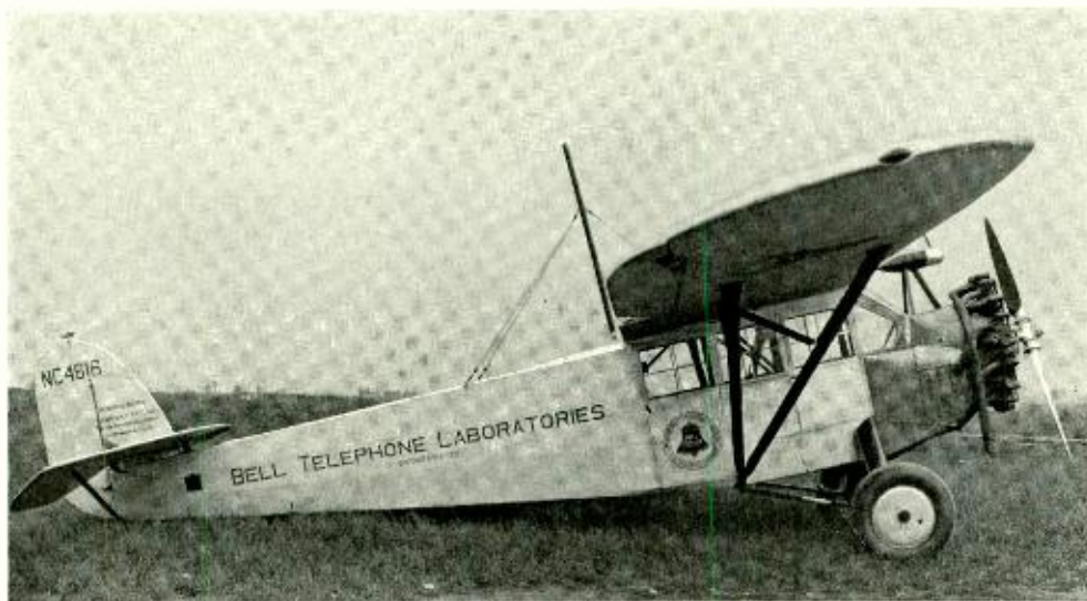
Fig. 1—The rod antenna and wind-driven generator may be seen in this photograph of the Laboratories' plane
