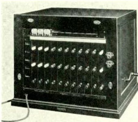
Fig. 1—Outer view of the 506-A switchboard. The other three pictures also show this switchboard
