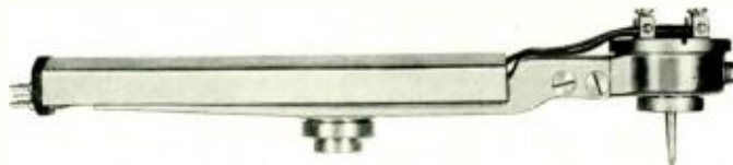
Fig. 6—Playback for reproduction directly from wax discs.
