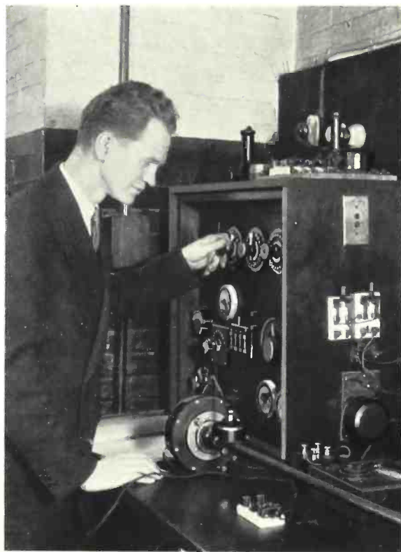
The 555-W Receiver is tested by connecting it to a long tube and measuring its input to this acoustic "line" by the condenser transmitter shown on top of the tube. Theodore Osmer had a large part in the development work
