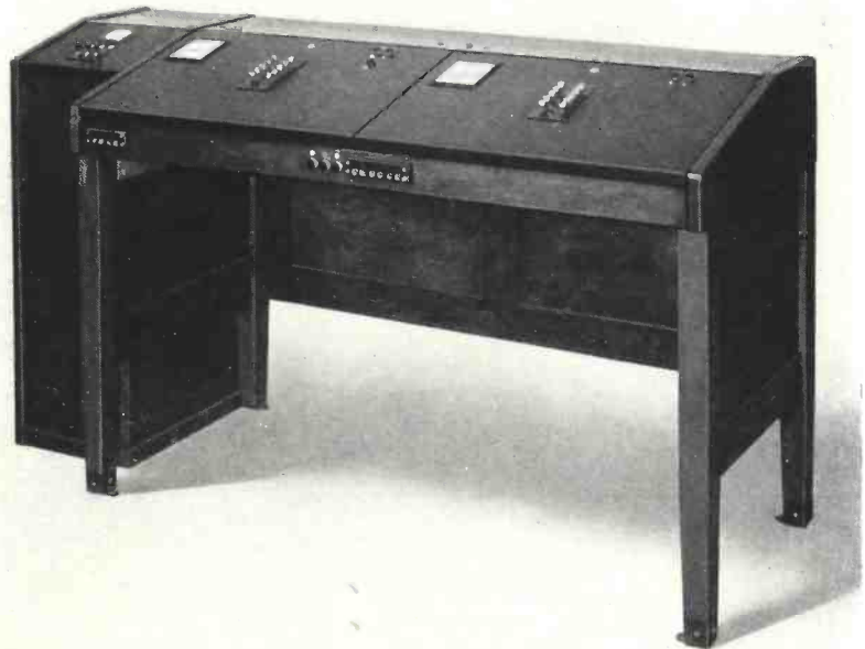
Two operators' positions. At the left is a section in which the cable comes up from the floor
