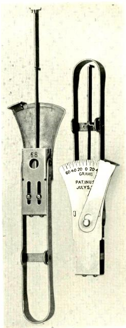
Pressure exerted by brushes in machine-switching devices is measured by this gauge. At the left it appears ready for use; at the right, with its handle folded to protect the reed when not in use. In the right-hand view is also seen the stop which facilitates repeated measurements
