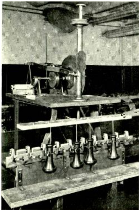
How receivers are tested in the dropping machine
