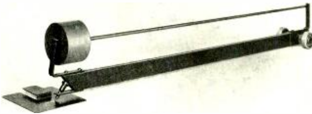
Testing a finish by moving the scratching point back and forth. The cylinder on the left is an adjustable weight
