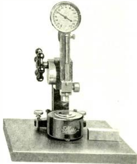
The scleroscope—another type of hardness tester
