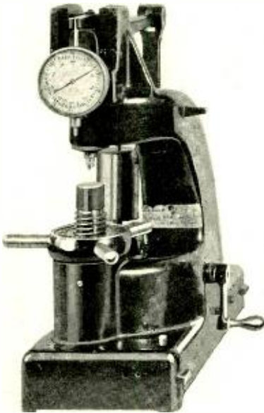
This Rockwell hardness test presses a steel ball into the sample
