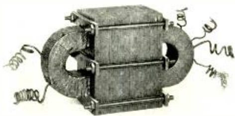
Fig. 3—Shell-type design of 1914; size 6 \frac{5}{8} by 4 inches
