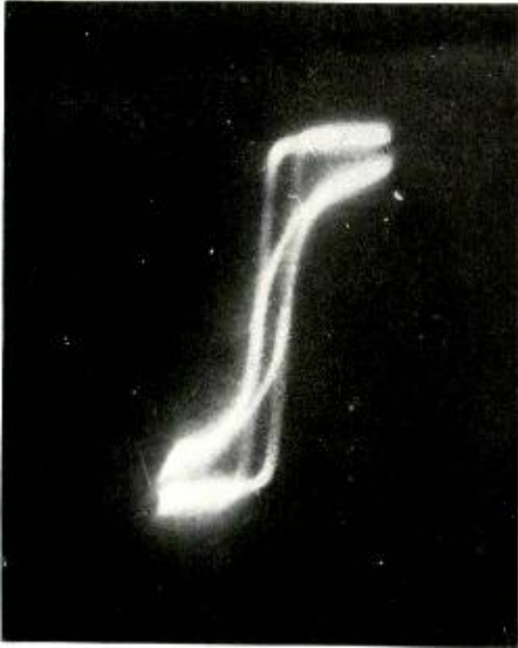
Hysteresis curves of permalloy (65% nickel, 35% iron), with and without tension
