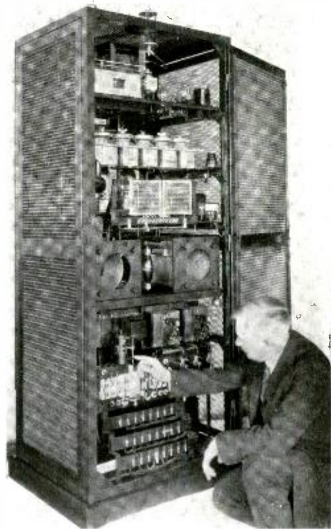
The author points out the flow-controlled relay in a 1000 watt broadcasting transmitter
