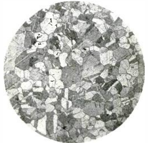
Fig. 3. The crystal structure of brass with its light and dark areas in many crystals, characteristic of this metal and known as "twinning." Magnification 85 times
