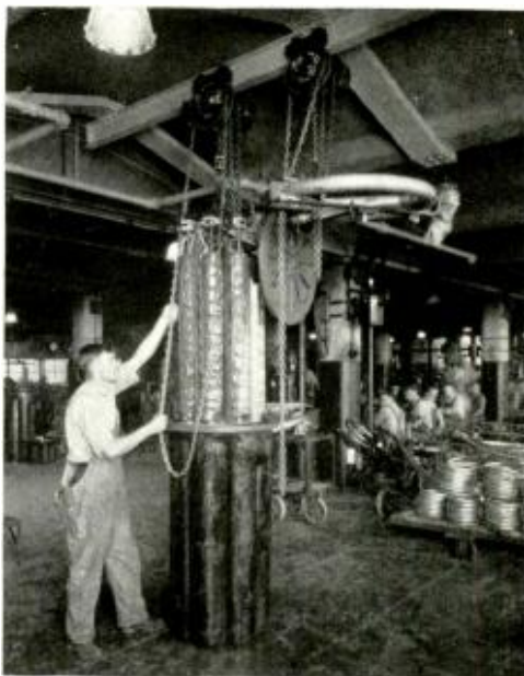
Final Assembly Operations; Lowering the Coil Assembly into the Case Casting
