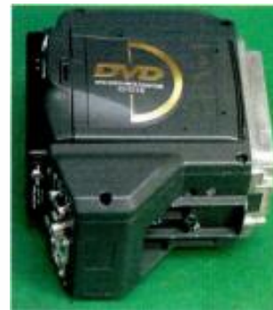
Hitachi has a DVD-RAM recording back for ENG cameras.
