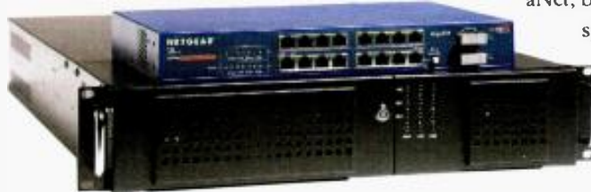
Avid's LANshare provides up to 640 GB of storage, holding 45 hours of content at DV25 resolution.
