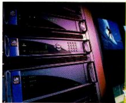
A look at S-A's Atlanta demo center, where 16 channels of programming are being compressed, distributed and received using (top to bottom) the PowerVu Plus encoder, Multiple Decryption Receiver and BitMizer statistical multiplexer. S-A's Explorer 2000 digital set-tops are partially visible.
