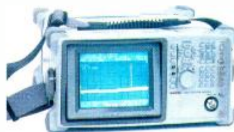
Tektronix’s new U3661 portable spectrum analyzer weighs only 24 pounds.
