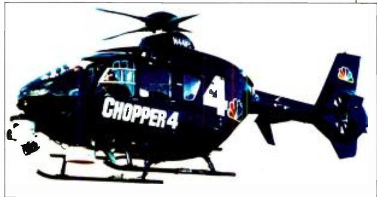
The new Chopper 4 has an enclosed tail rotor design that makes it 50% quieter than WNBC's old helicopter.
