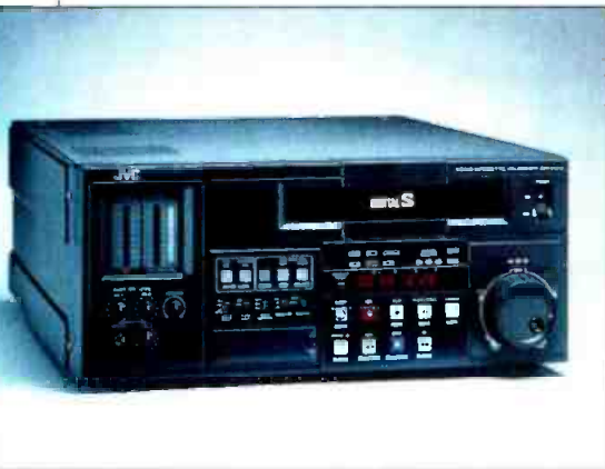
Memphis stations WPTY-TV and WLMT use the JVC BR-D80 Digital-S recorders to record ENG feeds and make A/B-roll edits.
