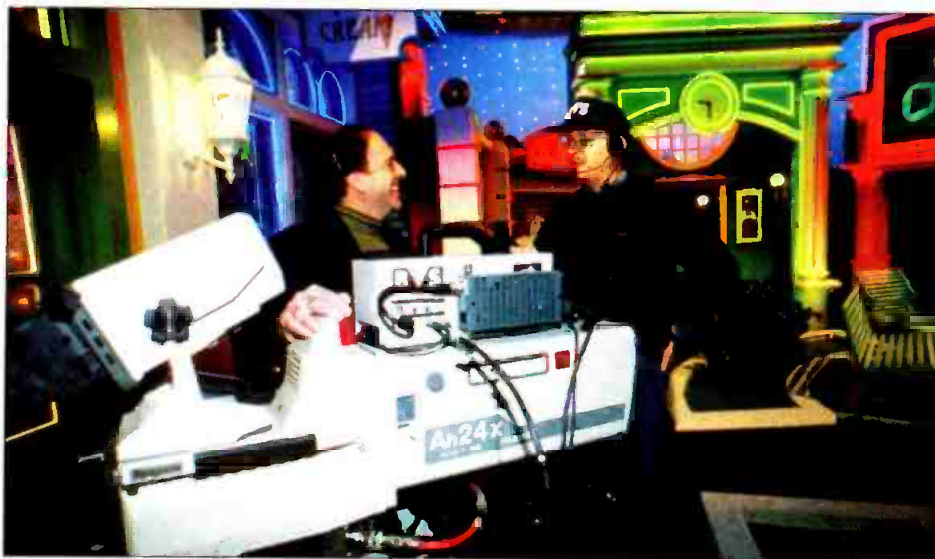
The show uses two sets of cameras, one with standard lighting and a second duplicating the setup with BVS (Beyond Visible Spectrum) equipment.
