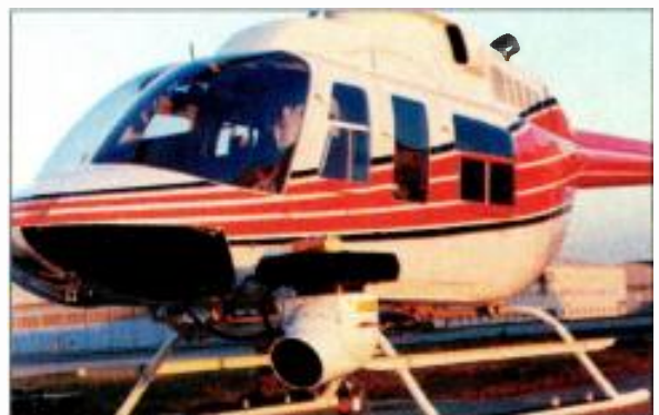
The Wescam 16SS-B750 gyrostabilized camera unit can be either nose- or side-mounted on a helicopter.
