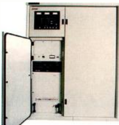
WRAL-HD is using a Harris Sigma CD transmitter with 8-VSB digital exciter.
