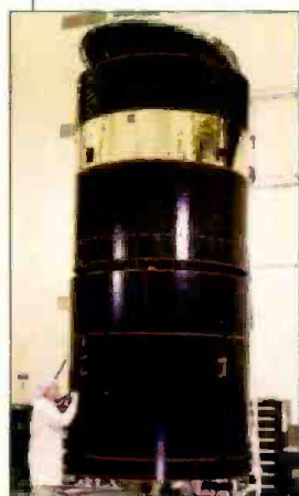
Hughes's Galaxy IX is a spin-stabilized HS 376 satellite that carries 24 16-watt C-band transponders.
