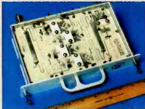
Silicon carbide transistor mounted in modules may be key to high-power solid-state UHF transmitters.
