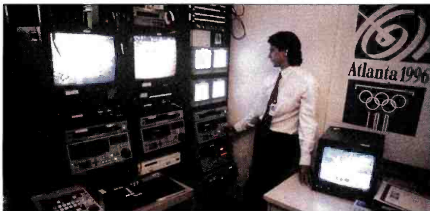
PAL and NTSC Panasonic D-3 systems duplicate video received from around the world in the dub room of the Atlanta Olympics production facility.
