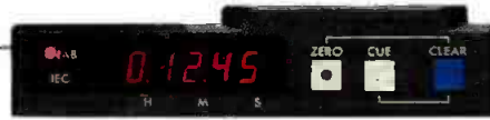
A built-in tape timer displays current tape position in hours, minutes, and seconds, and includes a search-to-cue locator with cue point and zero location memories.
