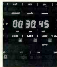
Timer-autolocator control panel
