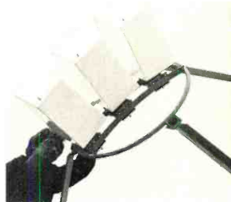
When installed on a 5-meter antenna, isolation between beams is better than 20 dB, with a loss of about 1 dB at 4° off boresight.
