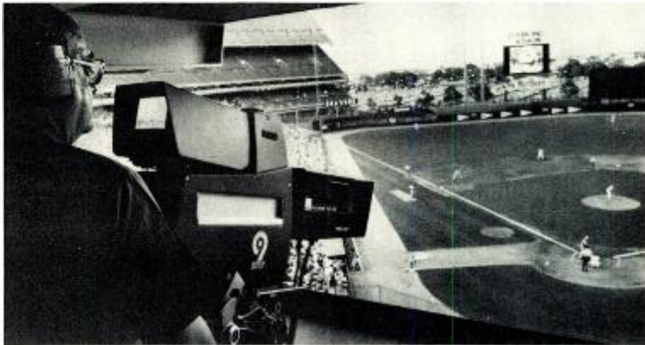
Channel 9 covers home plate action from one of their six TK-47 automatic color cameras. In the distance, the Met's Diamond Vision replays game action in slow motion from another TK-47 output.
