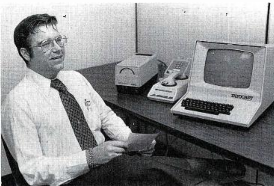
William VonMeister demonstrates (l-r) DBC’s DBT-1000 FM receiver-printer, a standard acoustical coupler and the EMS-300 message preparation device.
