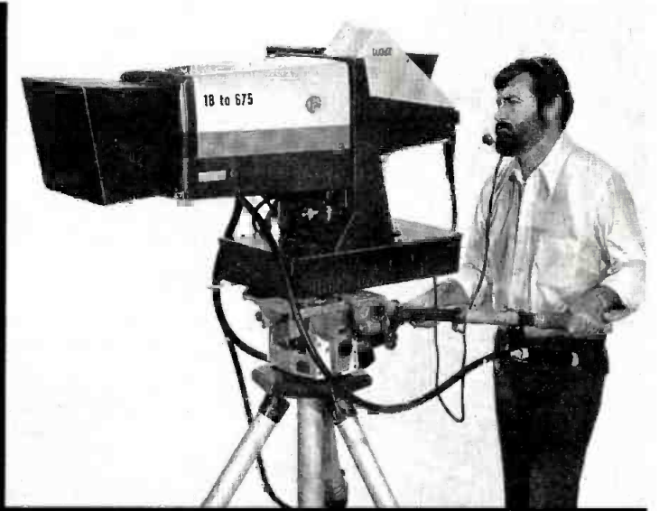
Studio camera conversion using Minimax adaptor.
