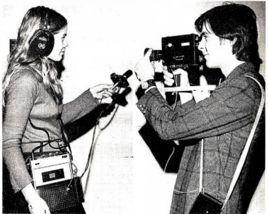
These are the two halves of MIT's prototype 8mm sync:sound system. The resulting pictures are said to have theater-sharp brilliance when used in TV transmission. Cost of both the sound unit (left) and the camera is expected to be under $1,000. Below: Jeremy Gury of Quadrant Communications, an ex-advertising agency executive, whose company will market the system.
