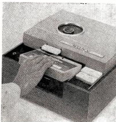
At a demonstration in New York last week Sony Corp. explained that loading a Videocassette into its home TV player was an easy, one-hand operation. The Videocassette provides a program up to 90 minutes.
