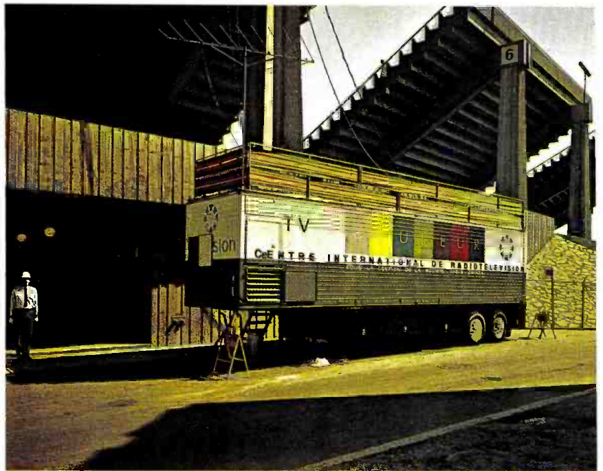
Air-conditioned RCA mobile unit built for CBC contained the control room for three-camera pickup.
