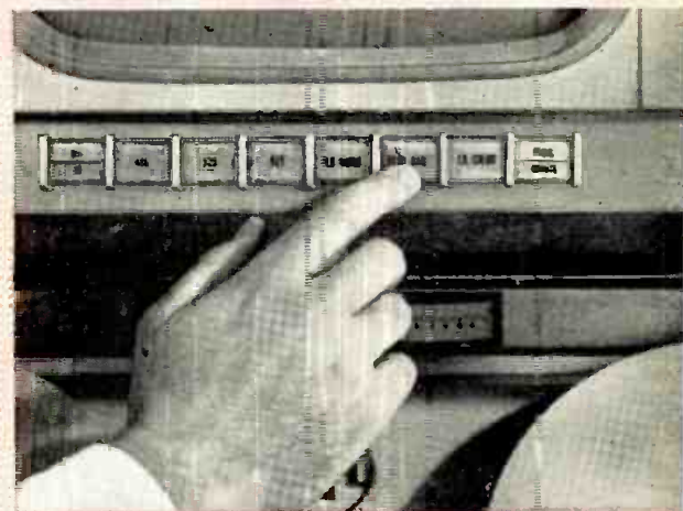
TR-70 has "instant selection" of high band or low band, color or monochrome.
