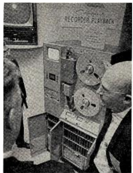
RCA showed three new TV tape recorders, including this TR-4, a solid-state record-playback unit.
