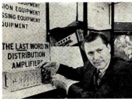
Module plug-in design of Dynair Electronics Inc.'s solid-state TV distribution amplifiers is exhibited by firm's George Bates.
