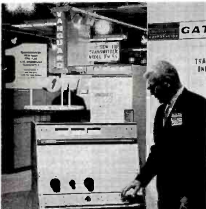
Not only unique one-tube design but also unusual styling mark Gates Radio Co.'s new Vanguard I 1-kw AM transmitter here demonstrated by firm's Reck Morgan.
