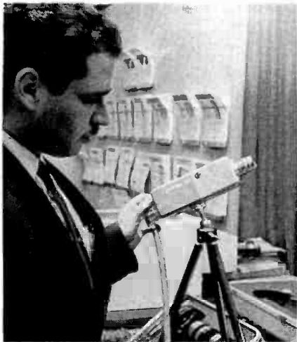
Miniaturized TV camera of Photo Research Corp. is operated by firm's Gideon Fiat. It weighs under 3 lbs.
