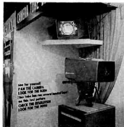
The new English Electric 3-inch image orthicon tube was shown mounted in Visual Electronic's Mark 10 zoom camera.
