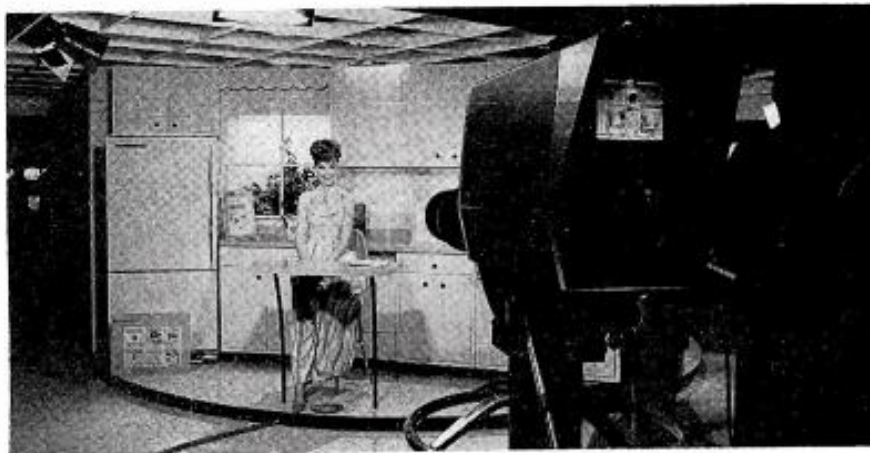
Sarkes Tarzian's new solid-state, zoom lens 3000L 3-inch image orthicon camera
