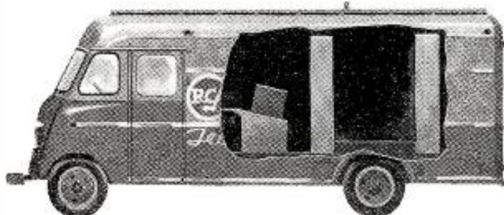
Mobile unit arrangement—accommodating cameras and tape equipment in one place.
