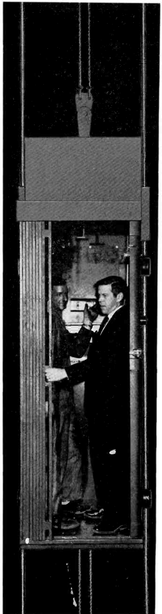
(right) Rated for a load of 750 pounds, will comfortably accommodate two people. Car stops automatically if door is opened, will not start until it is closed. Supported by a double set of cables, either one of which will hold the car and its full load.
