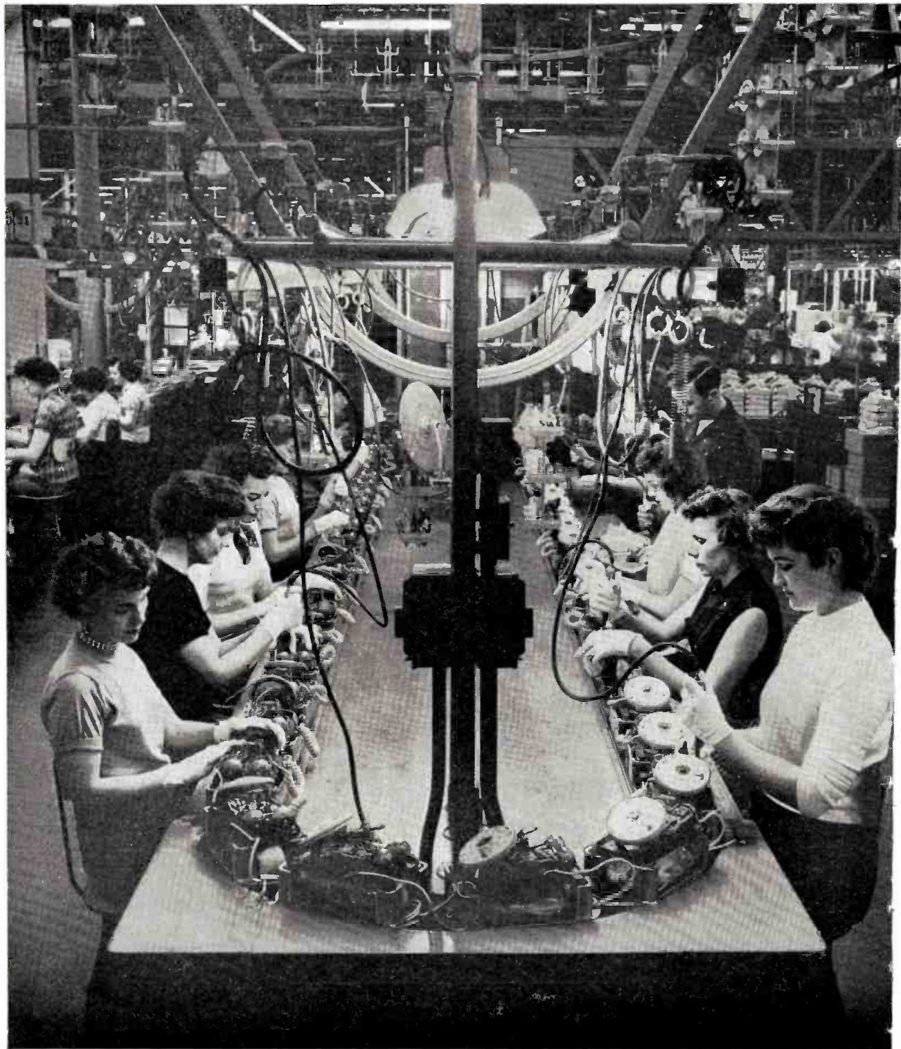
TELEPHONE TEAMWORK. At Western Electric's Indianapolis Works, these girls handle the final assembly of telephone sets. A 2½-mile long conveyor system links the various manufacturing steps, bringing components and sub-assemblies from every corner of the plant.
