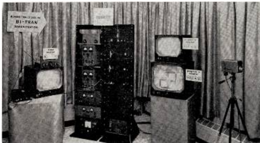
BI-TRAN system of tv broadcasting was demonstrated last week by Blonder-Tongue Labs., Newark, N. J. Bi-Tran is designed to permit the telecasting of two programs simultaneously on the same channel. The company believes the system has applications for the military, government, industry and educational groups.
