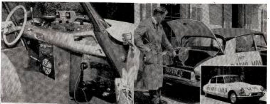
THIS is the custom-designed mobile unit used by Radio Monte Carlo for remote recording assignments. Basic ingredients are an Ampex 600 recording unit and a Citroen 19 automobile. The Ampex machine has been built into the dashboard (cut at left) for convenient operation by the driver. Other accessory equipment is arranged compactly within the driver's reach. Even the trunk is used to full advantage: note the microphone cord and power cables mounted on reels in the picture at right.
