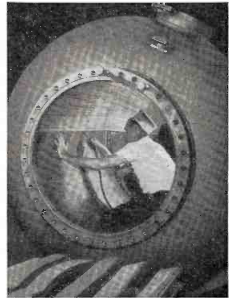
2 Million Volts will be generated in this all-steel transformer tank. It is part of an x-ray machine used for industrial inspection. USS steel plates and sheets were used for the important parts.
