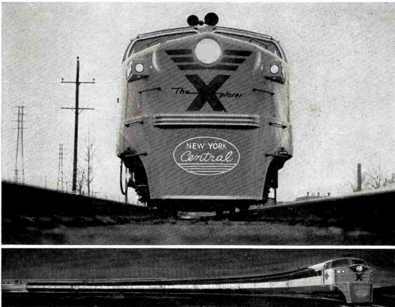
The glamour-coach Xplorer is 2½ feet lower, faster, more comfortable, more economical to build and operate than trains of present-day design
