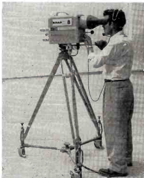
NEW five-inch view-finder studio camera with four-lens turret will be shown by Kay Lab. Camera has rear turret control with side-handle focus.
